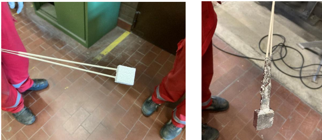
Figure 116: AISCAN probes before (left) and after use (right)
