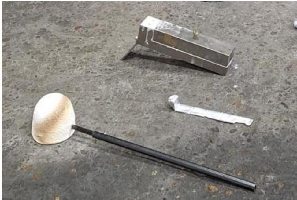
Figure 12: K-mold test equipment and obtained samples.
