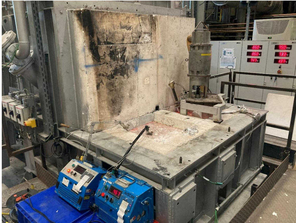
Figure 115: Setup for hydrogen pickup measurements: external chamber divided into a pump (right) and into a sampling chamber (left)
