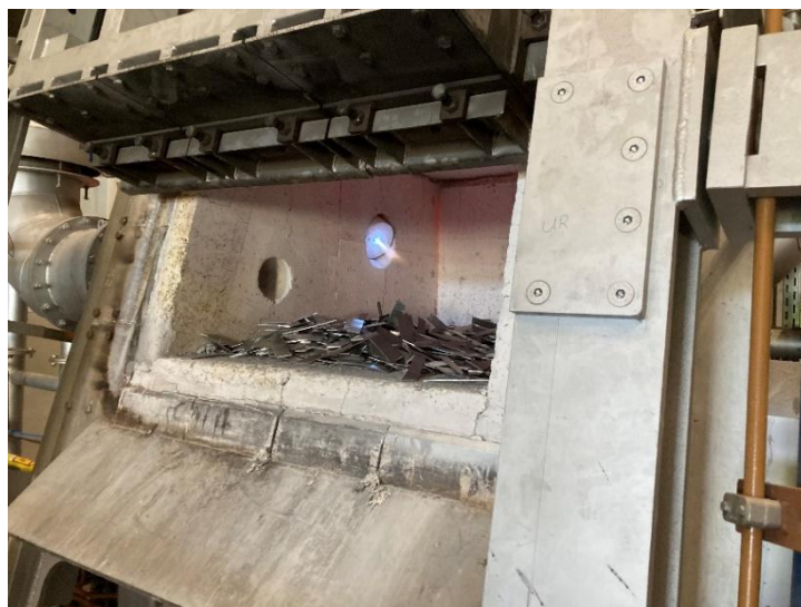
Figure 105: Loaded furnace with pilot flame switched on
