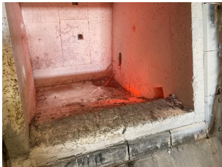
Figure 110: All metal has melted; the bath thermocouple is immersed in the melt at the rear right
