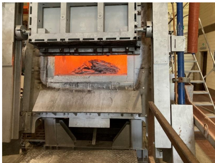
Figure 108: Preheated furnace fully charged with trimmings
