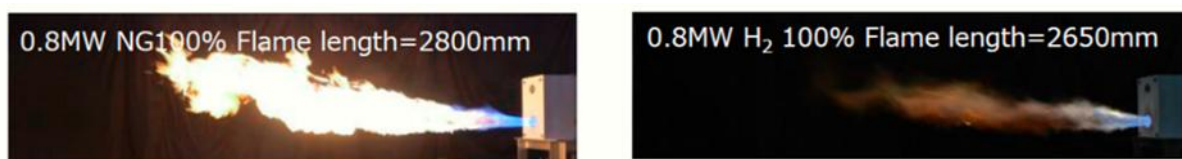
Figure 58: Flame length of an oxyfuel burner
