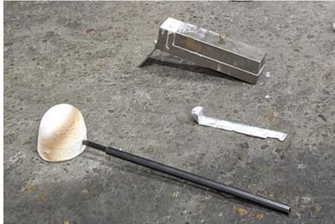
Figure 36: K-mold test equipment and obtained samples.
