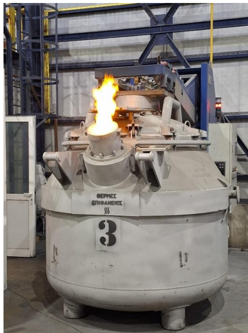
Figure 10: Test with H 2 +O 2 in crucible #3.
