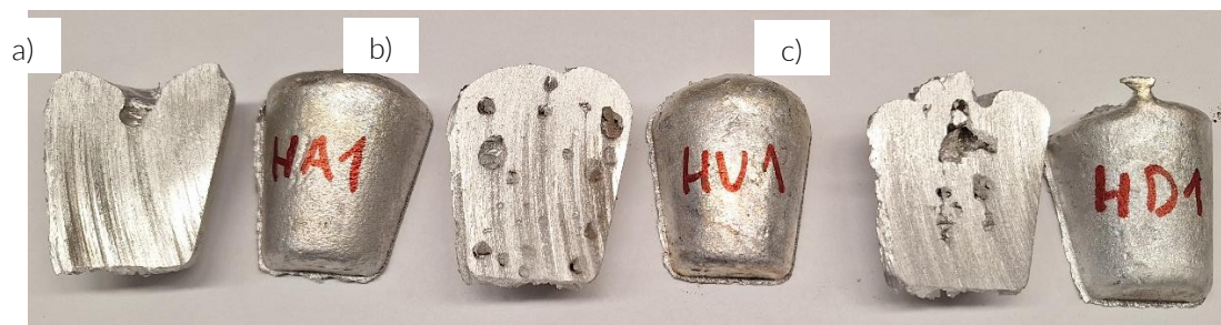
Figure 15: Example of test samples obtained in the vacuum and dross test: a) Air; b) Vacuum; c) Dross.
