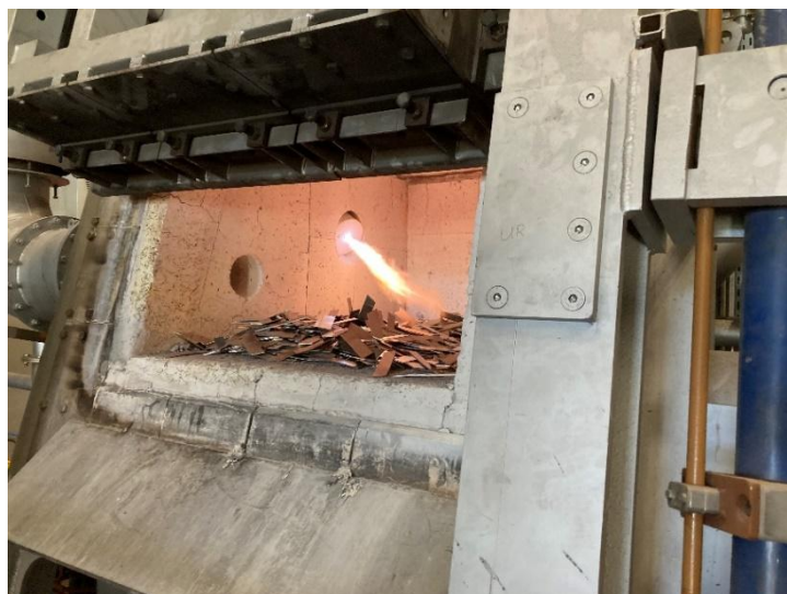
Figure 106: Burner flame switching to normal mode
