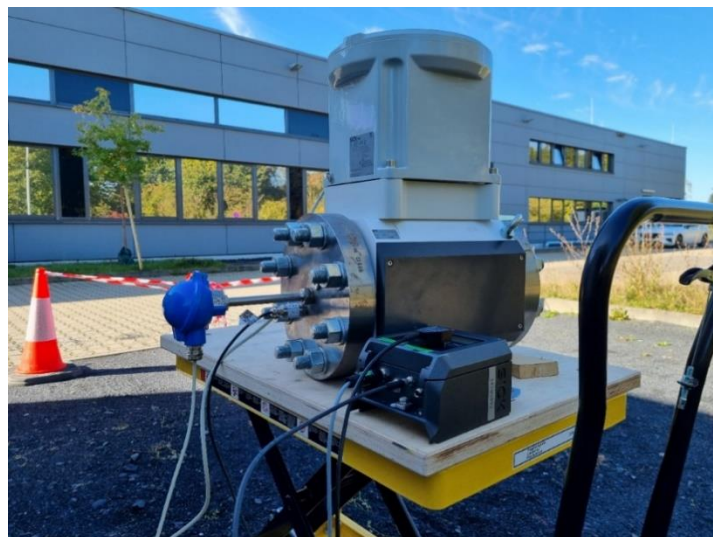
Figure 25: 4" SICK Prototype USM for H 2 measurements.
