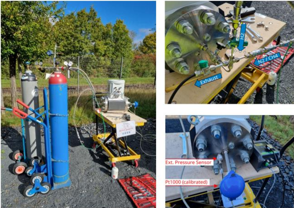
Figure 26: Test setup for H 2 purity measurements at SIEN.
