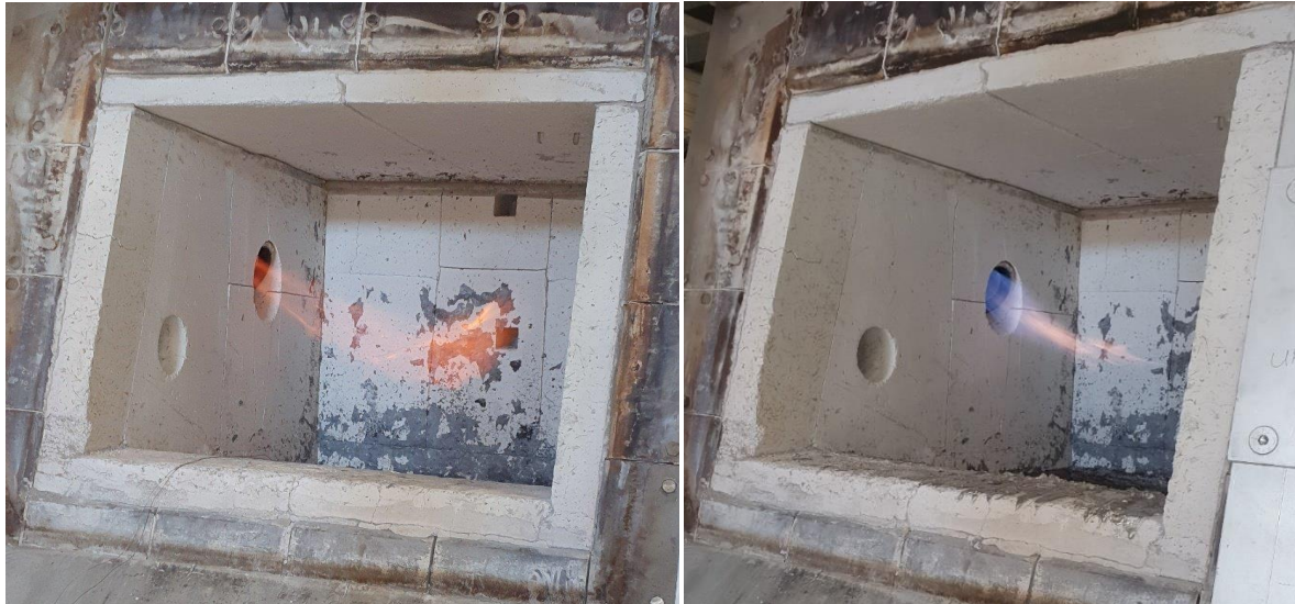
Figure 19: Flame appearance hydrogen-air (left) versus natural gas-air (right)
