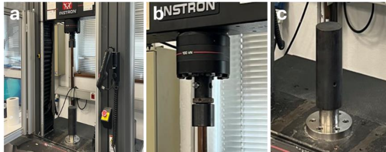
Figure 52. a. Instron 5982 - resilience test setup; b. Upper tooling; c. Lower tooling.
