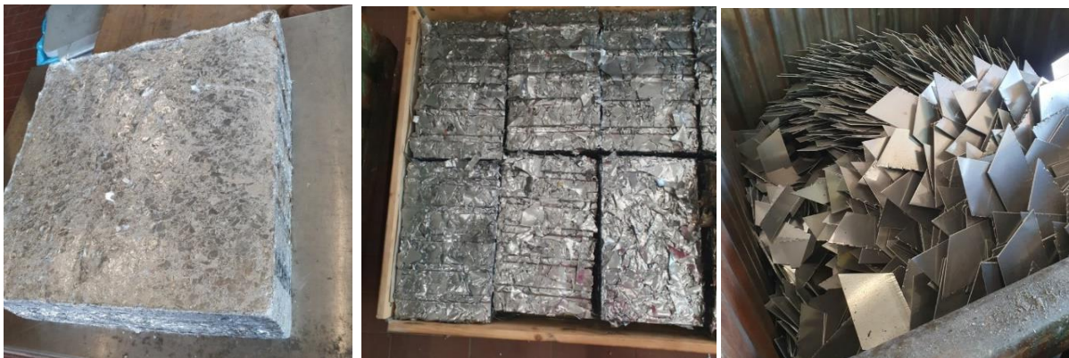
Figure 21: Baled foil scrap (left) and can body stock (cbs) stampings (middle) and trimmings of can lid stock (right).
