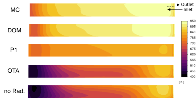
Figure 3- 4 Wall temperature profile along the active cooling tube.
