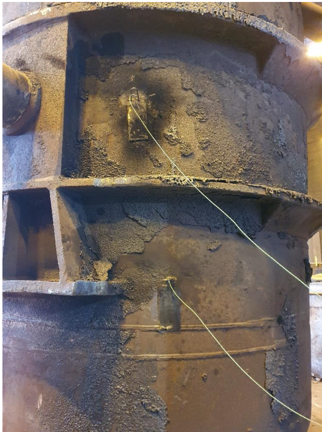
Figure 134. Photo of the two thermocouples in the ladle wall
