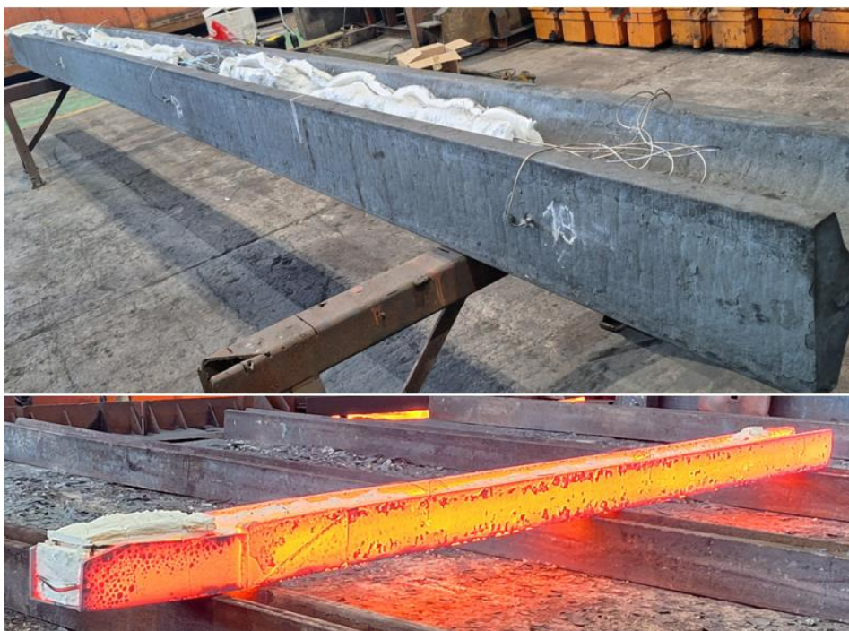
Figure 40. Monitored BB2 before and after entering the reheating furnace of AMOB.
