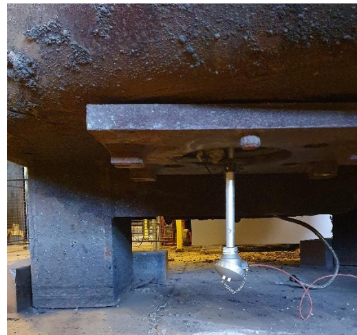
Figure 136. Photo of the thermocouple inserted through the tapping hole.
