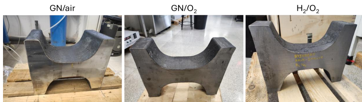
Figure 72. Beam blanks 2 produced in AMOB under NG/air, NG/O 2 and H 2 /O 2 combustion programme with the two new burners.
