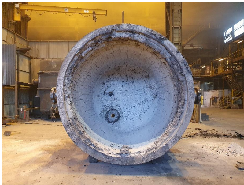
Figure 127. View inside the ladle used in the demonstration. The worn refractory visible.
