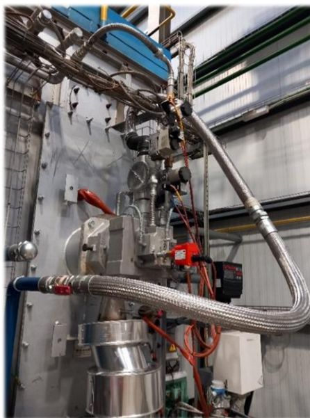
Figure 197. Self-recuperative burner and position of the thermocouples along the radiant tube (right).
