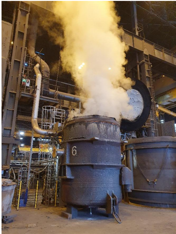
Figure 145. A condensation cloud above the ladle heater shortly after start-up of the hydrogen test.
