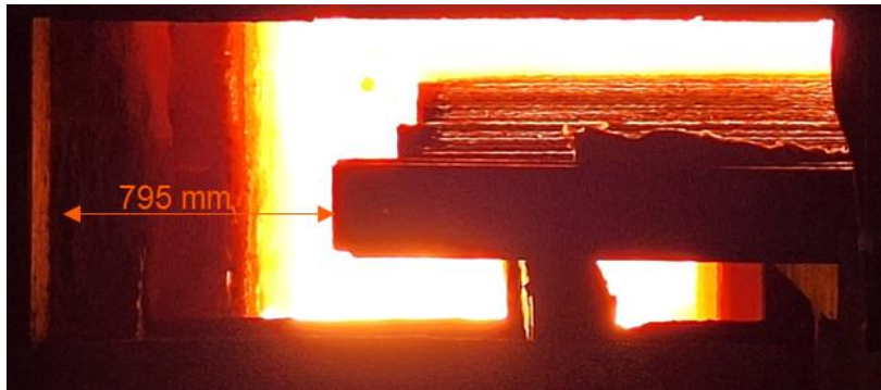
Figure 39. BB2 at the entrance of the furnace, positioned on the beams.
