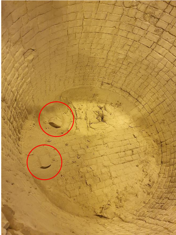
Figure 141. A Pentabrick C01 and Sindoform K40 sample in the prior to the hydrogen test.
