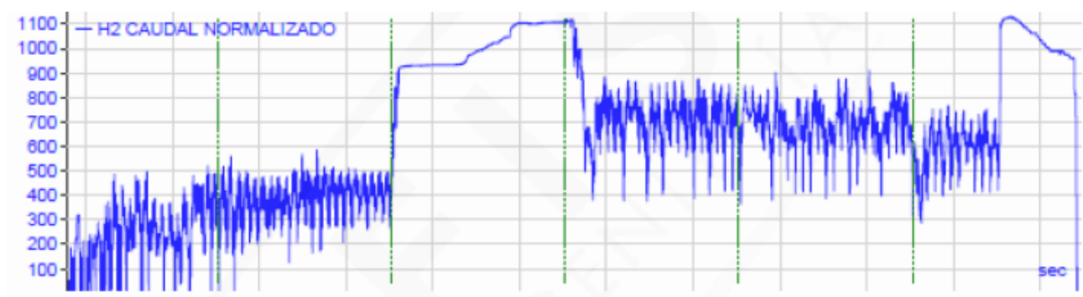
Figure 12. H2 flow rate during TEST 2.
