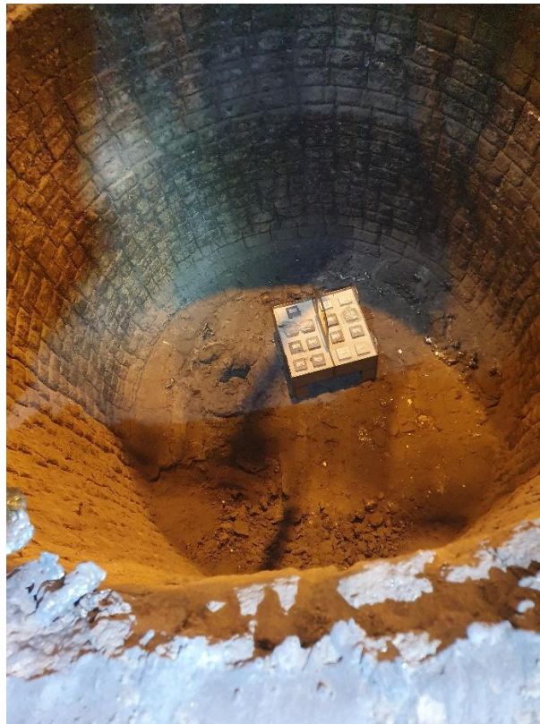
Figure 140. The refractory sample box inside the test ladle prior to the heating with CO-mix gas.
