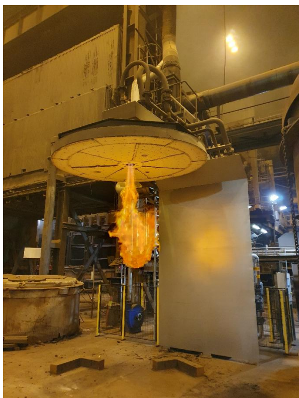
Figure 143. Photo of the flame during testing in hydrogen-air combustion mode.
