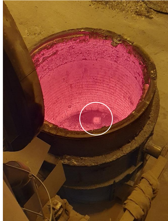
Figure 142. One of the two refractory samples visible after the hydrogen test.
