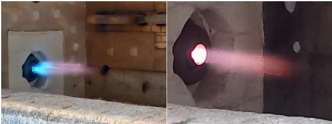
Figure 12. Burner start up with NG (left) and H 2 (right)..
