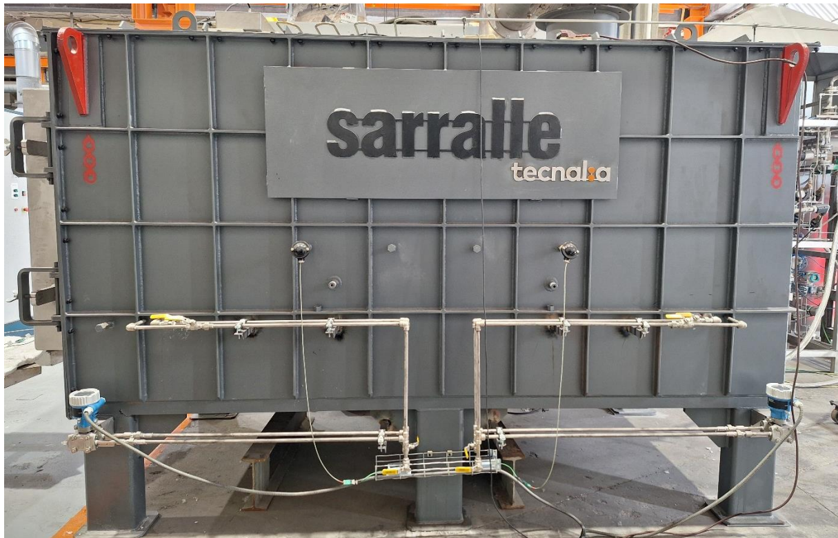
Figure 16. Combustion chamber with the differential pressure transmitters.
