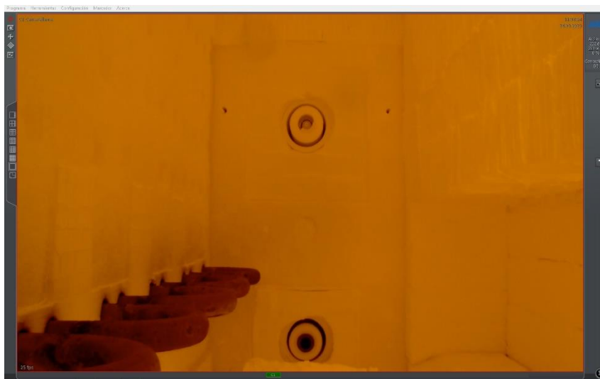
Figure 13. Flameless operation at operating temperature with hydrogen.
