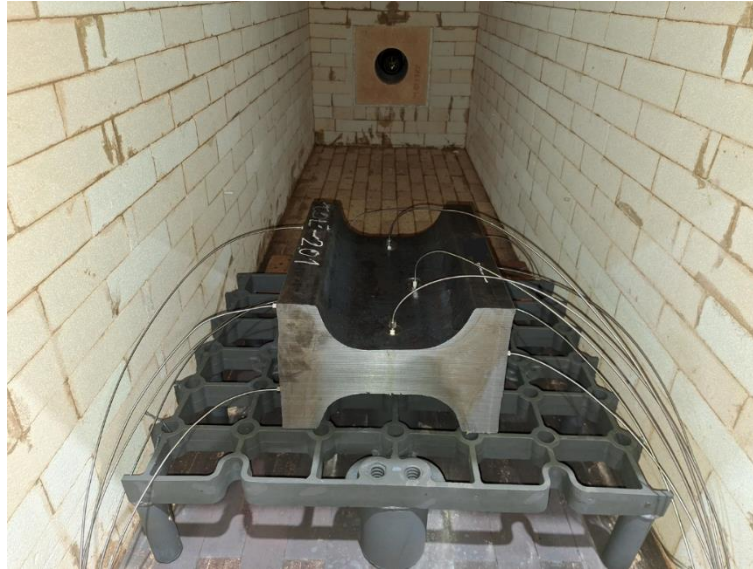
Figure 19. Structural steel sample with 11 thermocouples inside the combustion chamber.
