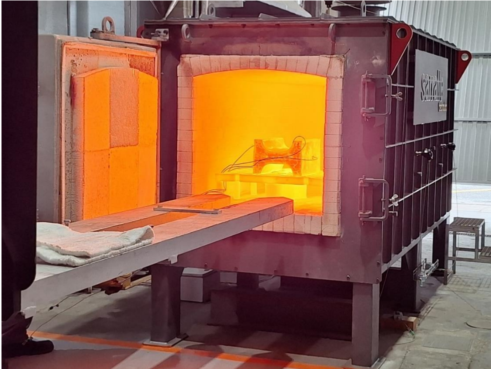
Figure 26. Picture of the sample inside the combustion chamber prior to unloading it.
