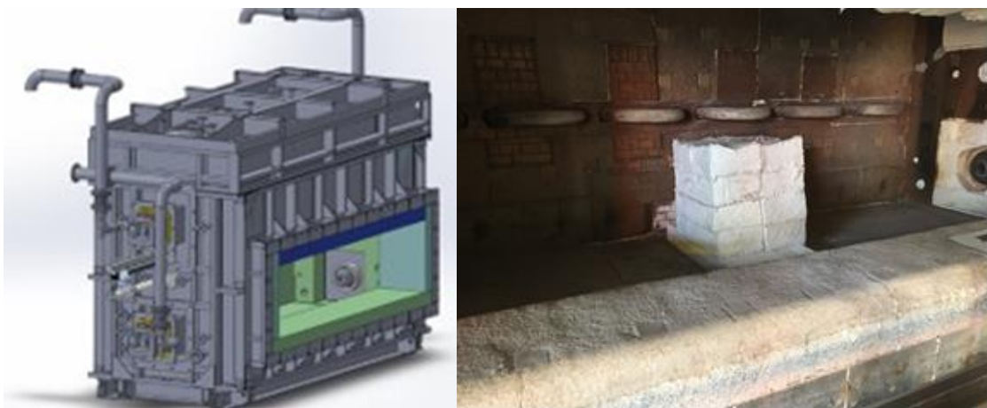
Figure 11. Sestao burners integration at AMI furnace for preliminary trials.
